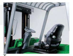
I he roomy, comfortable, ergonomic driving seat is easily accessible thanks to the large, convenient step. The masts are designed for excellent visibility and unrivalled safety thanks to their torsional rigidity and stability at the maximum height.
