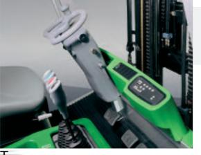
I he operator selects the driving programs (L - H - P) easily by just pressing the buttons on the steering column. The automotive-style dashboard, with alphanumeric display, allows easy identification of diagnostic codes. In the standard version, it also carries travel direction and driving program indicator lights and the electronic hour counter.
