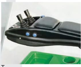
he proportional electronic controls integrated in the new (optional) armrest enable the operator to manage all the hydraulic functions by simply moving the Mini-Joystick or Fingertips levers. The inversion of the drive direction is managed by the simple touch of the buttons placed on the driver's armrest.
