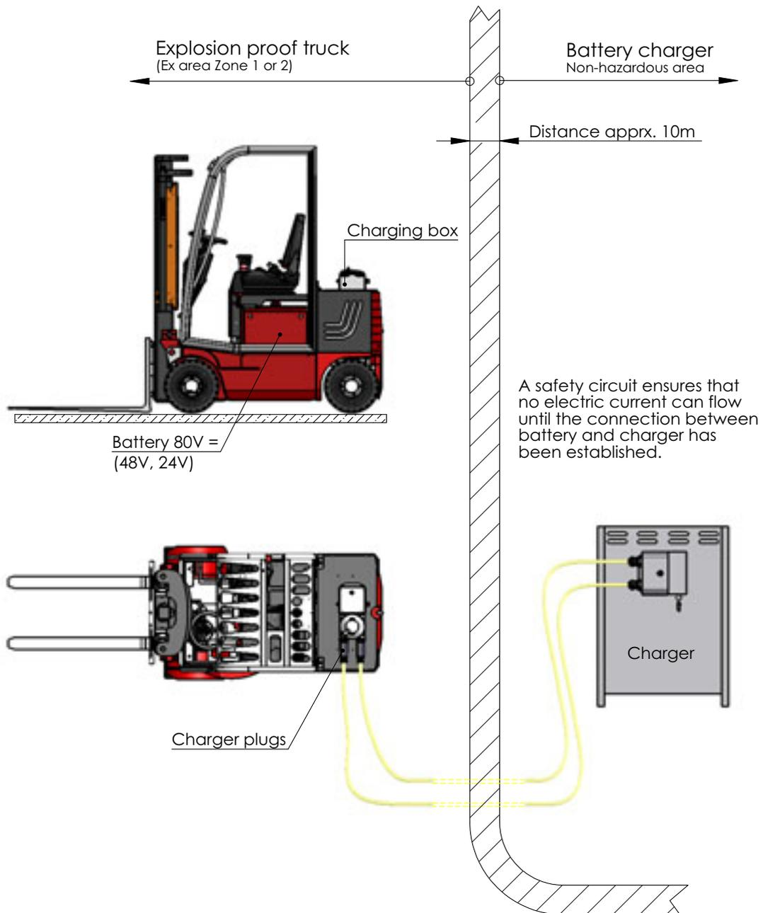
By releasing the safety screw, a contactor automatically breaks the electric flow and then the charging plugs may be safely removed from their sockets.
