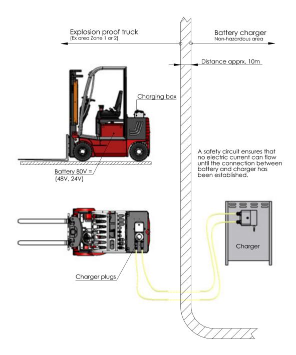
By releasing the safety screw, a contactor automatically breaks the electric circuit and then the charging plugs may be safely removed from their sockets.
