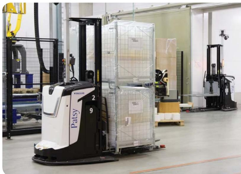
“instead of two AGVs, we now have six of them. As we work in three shifts, using AGVs helps us in cutting the material handling costs significantly. It is easy to understand that a similar non-automated transport system would require a lot of people to drive the forklift trucks.”
