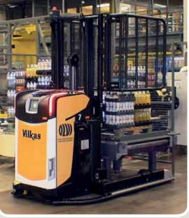
The Finnish brewing and soft drinks company Olvi acquired its brewery an automated warehouse truck solution from Rocla. Olvi was looking for cost savings by automatizing the basic transfers in the storage and picking areas. The automated solution is based on innovative, internationally awarded automated warehouse truck concept developed by Rocla.
